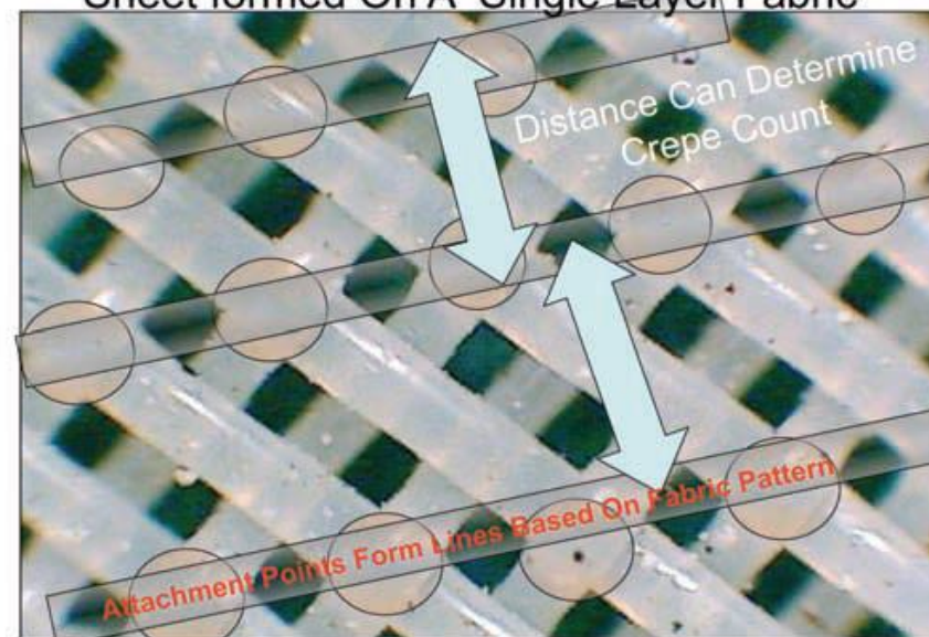
View Of Coating Attachment Points Of A Sheet formed On A Single Layer Fabric
